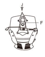
Using mechanism screws (J) to fix the mechanism (D) on the seat cushion(G). Tighten the screws with the enclosed Allen Wrench (N).
