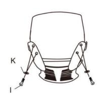
Using Seat amrest screws (I) and washers (K) to fix the armrest (E) on the seat cushion (G). Tighten the screws with the enclosed Allen Wrench (N).
