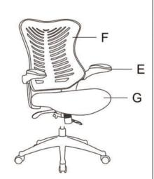
Now put the assembled back, seat and mechanism on to the assembled gas lifter. Push down firmly until the connection is ensure
