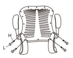
Using Back amrest screws (H) to fix the amrest (E) on the back cushion (F). Tighten the screws with the enclosed Allen Wrench (N). Put the amrest cover (L) on the amrest holes.
