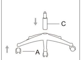
Press the Casters (A) into the holes at the end of each leg of Base(B). Insert the bottom end of the gas lifter (C), into the center hole of the base (B). Slide the gas lifter cover (M) onto the gas lifter (C)
