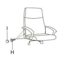
Using the armrest screws (H) to fix the armrest (E) on the back cushion (F) and seat cushion (G). Tighten the screws (H) with the enclosed Allen Wrench (K).
