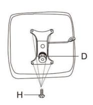
Using the Screws(H) to fix the mechanism (D) on the seat cushion (G). Tighten the screws (H) with the enclosed Allen Wrench (K).
