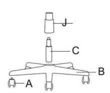
Press the Casters (A) into the holes at the end of each leg of Base(B). Insert the bottom end of the gas lifter (C), into the center hole of the base (B). Put the Gas lifter cover (J) on the gas lifter.
